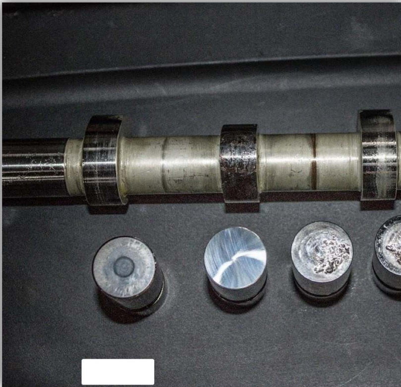
Unserviceable cam and lifters due to scaling
