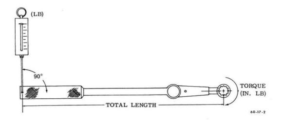
Computing Torque with Spring Scale Figure 202
