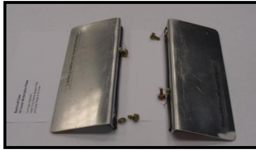
Figure 4: Oil Cooler Baffles, Photo by Ray Assmar
