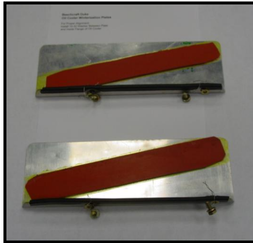
Figure 5 Oil Cooler Baffles, Photo by Ray Assmar
