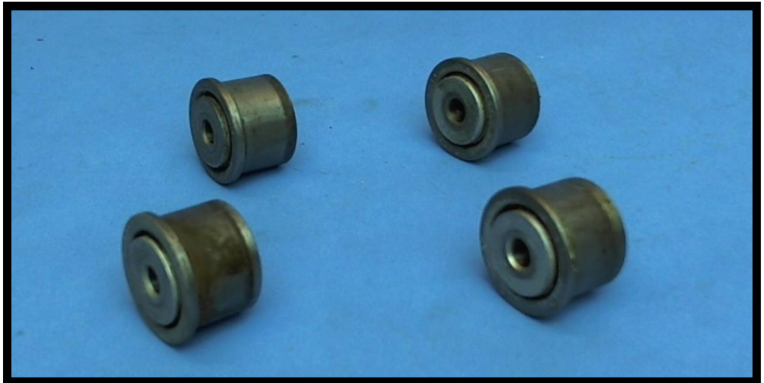
Figure 5. B60 Flap rollers, photo by Texas Air Salvage
