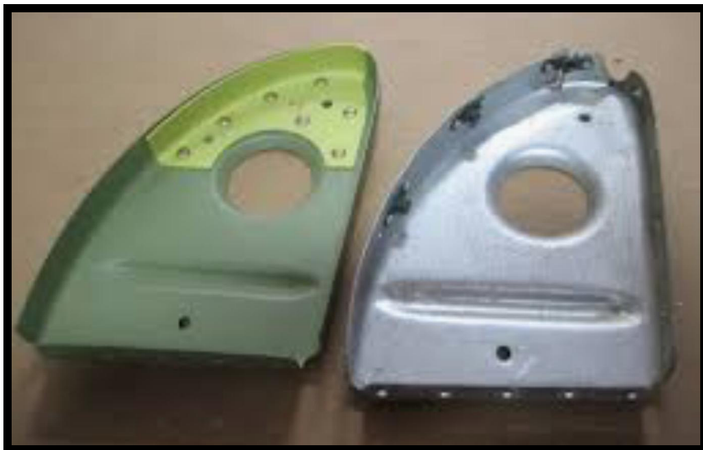
Figure 9. Cracked nose rib, Special Airworthiness Information Bulletin SAIB CE 11-21
