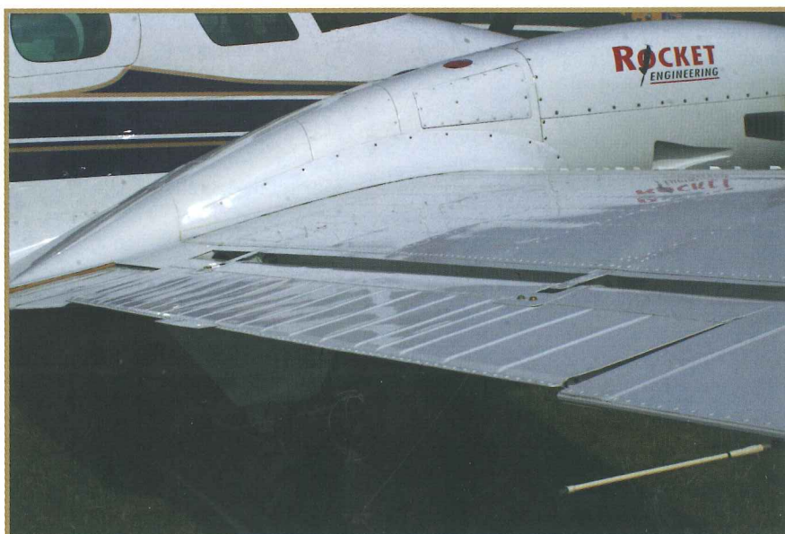
The Duke wing featured extended-chord flaps and a generous aileron gap.
