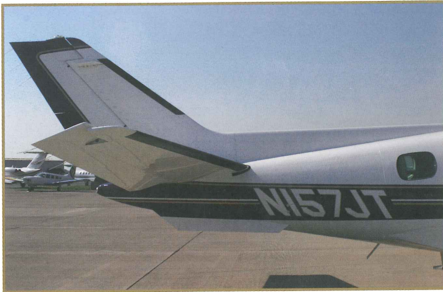
The Duke empennage sets it apart from any other Beechcraft; the strakes under the tailcone are an aftermarket add-on to enhance damp yaw response.
