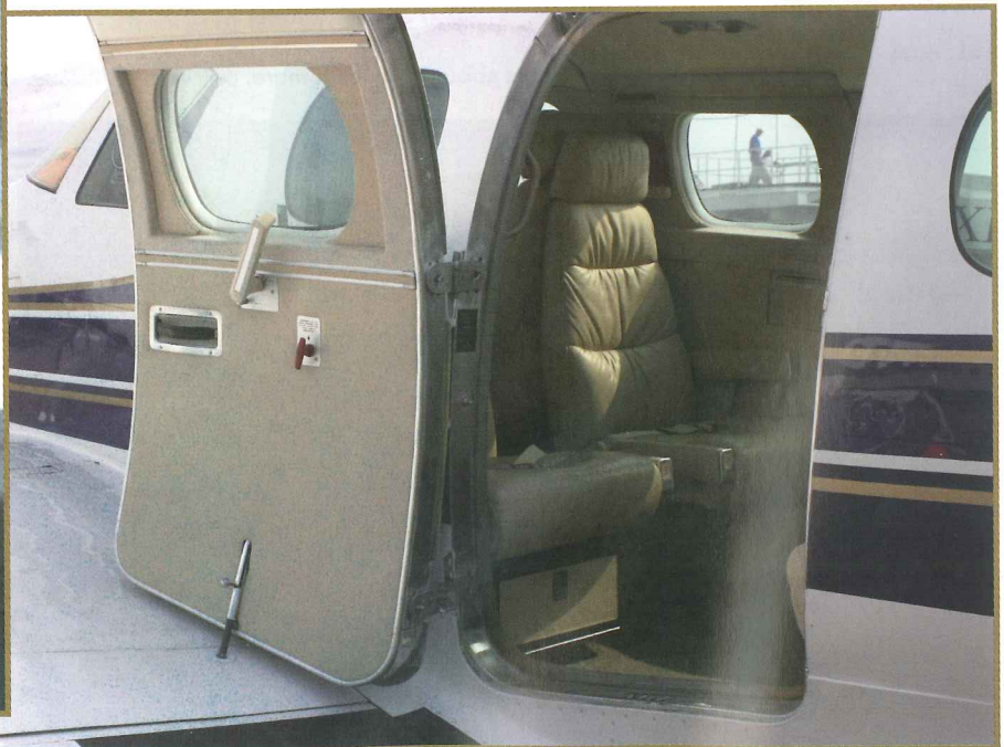
Boarding the Duke cabin is a two-step affair onto the wingwalk, using the Rocket Engineering-designed handles.
