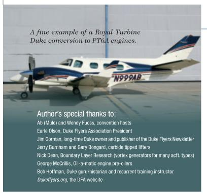
A couple of electrical gremlins were put to rest with an alternator conversion, lightweight starters and the change to a lead acid battery instead of the original NiCad. Vortex generators should be mandatory on all twins and you will find them on most Dukes. Their effect on performance allows not only a gross weight increase, but single engine flight to near stall speed. The two 380-hp turbo Lycomings like fuel, and lots of
