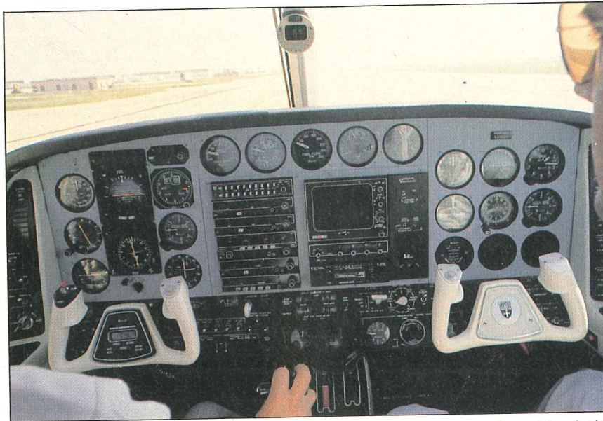
The Beech Duke features an uncluttered instrument panel that is nicely configured for single-pilot operations. This Beech demonstrator is equipped with King Radio's latest panel-mounted package, including its new KWX 56 stabilized radar.
